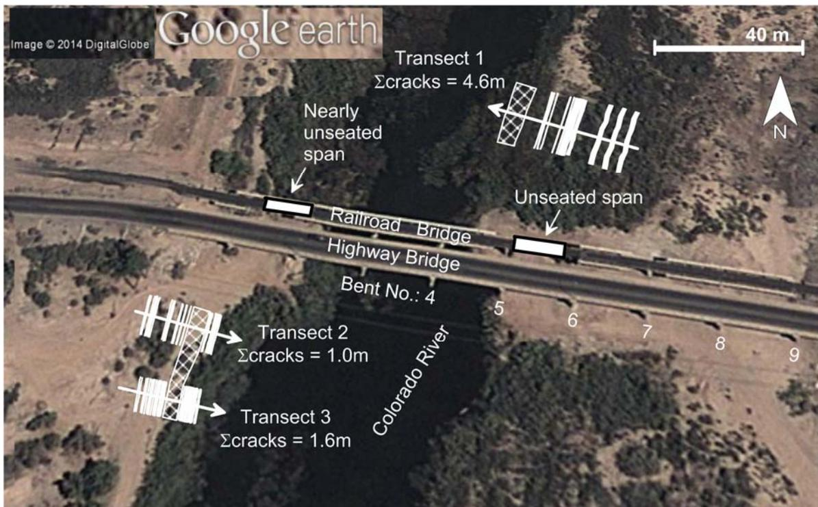
Figure 1: San Felipe Bridges site showing locations of structural damage and mapped ground failures following the 2010 El Mayor-Cucapah earthquake (after GEER, 2010).
