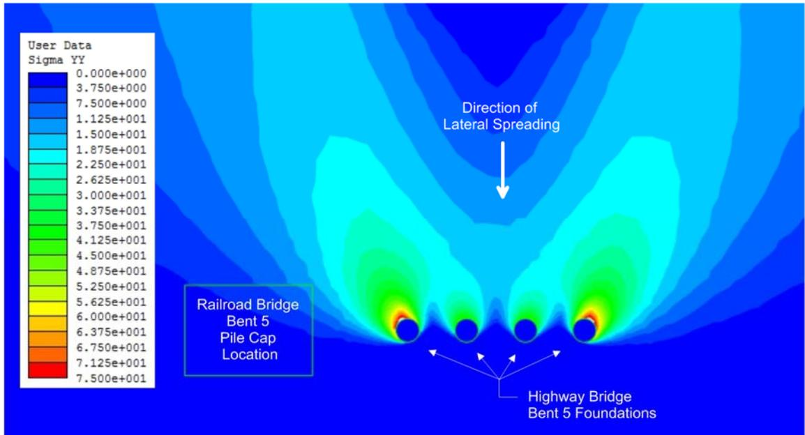
Figure 3: Results of Bent 5 finite element simulations with 4 m of imposed lateral spreading displacement, showing normal stress acting in direction of lateral spreading. Note arching between highway bridge foundations. Stress contours in kPa.
