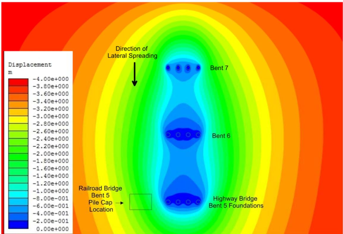
Figure 4: Displacement results (in meters) for finite element model including Bents 5, 6, and 7 of the highway bridge showing approximately 50 percent reduction in displacement at location of railroad bridge Bent 5 compared to free-field lateral spreading displacement of 4 m.
