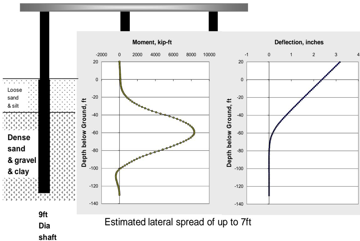
**Figure 3** Computed Lateral Bending Moments and Deflections for Lateral Spreading
