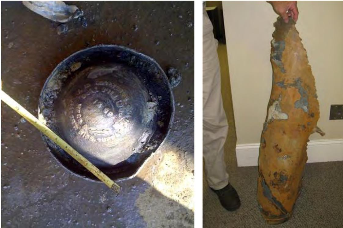
**Figure 8** Portions of Steel Piling Removed from Drilled Shaft Excavations
