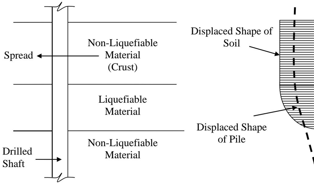
**Figure 2** Schematic Diagram of Lateral Spreading
