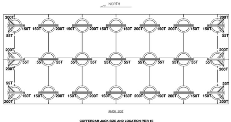
Figure 6. Plan View, Typical Pier Jack Layout
