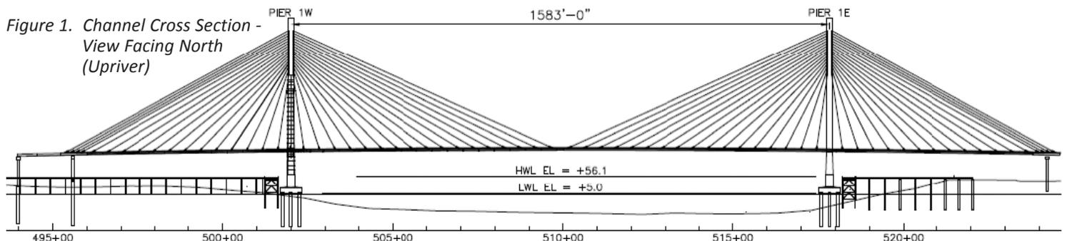
Figure 1. Channel Cross Section - View Facing North (Upriver)
