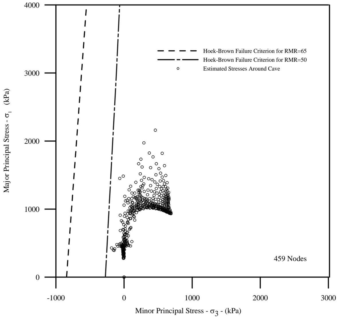
FIG. 2. Estimated Stress Conditions for Model 1 - Long Narrow Inclined Cave
