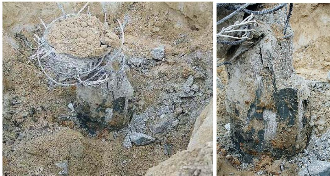
Figure 6 Broken Top of Shaft after Load Test
