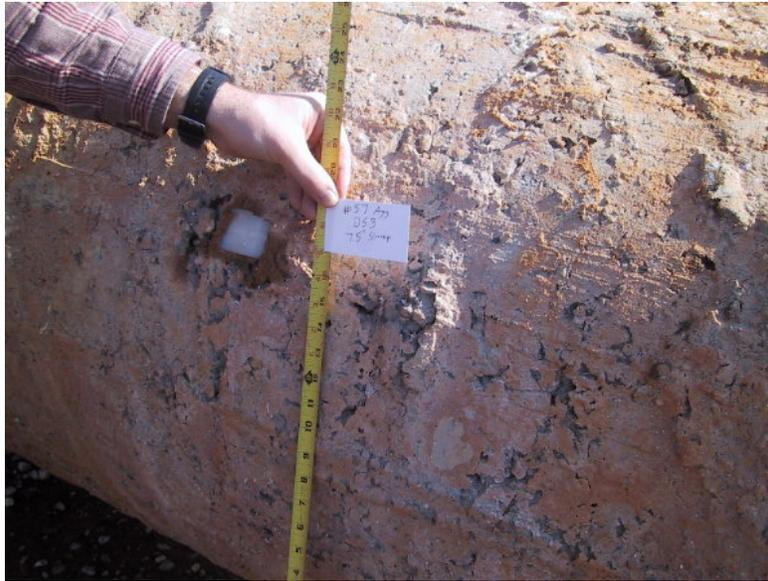
Figure 2 Surface of the Shaft with #57 Stone
