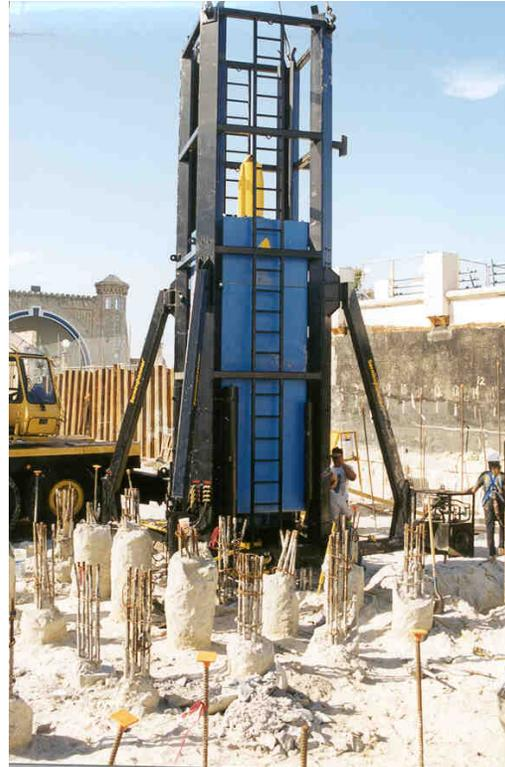
**Figure 6 Proof Testing of Production Piles with Statnamic (Rapid Load Test) Device at a project in Florida**
