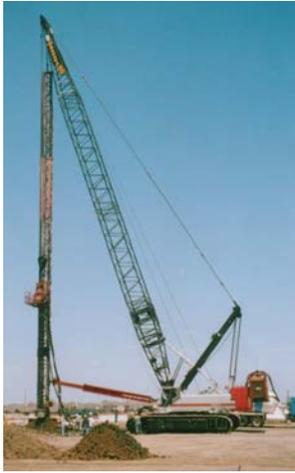
**Figure 1 Crane Attachment for ACIP Pile**
