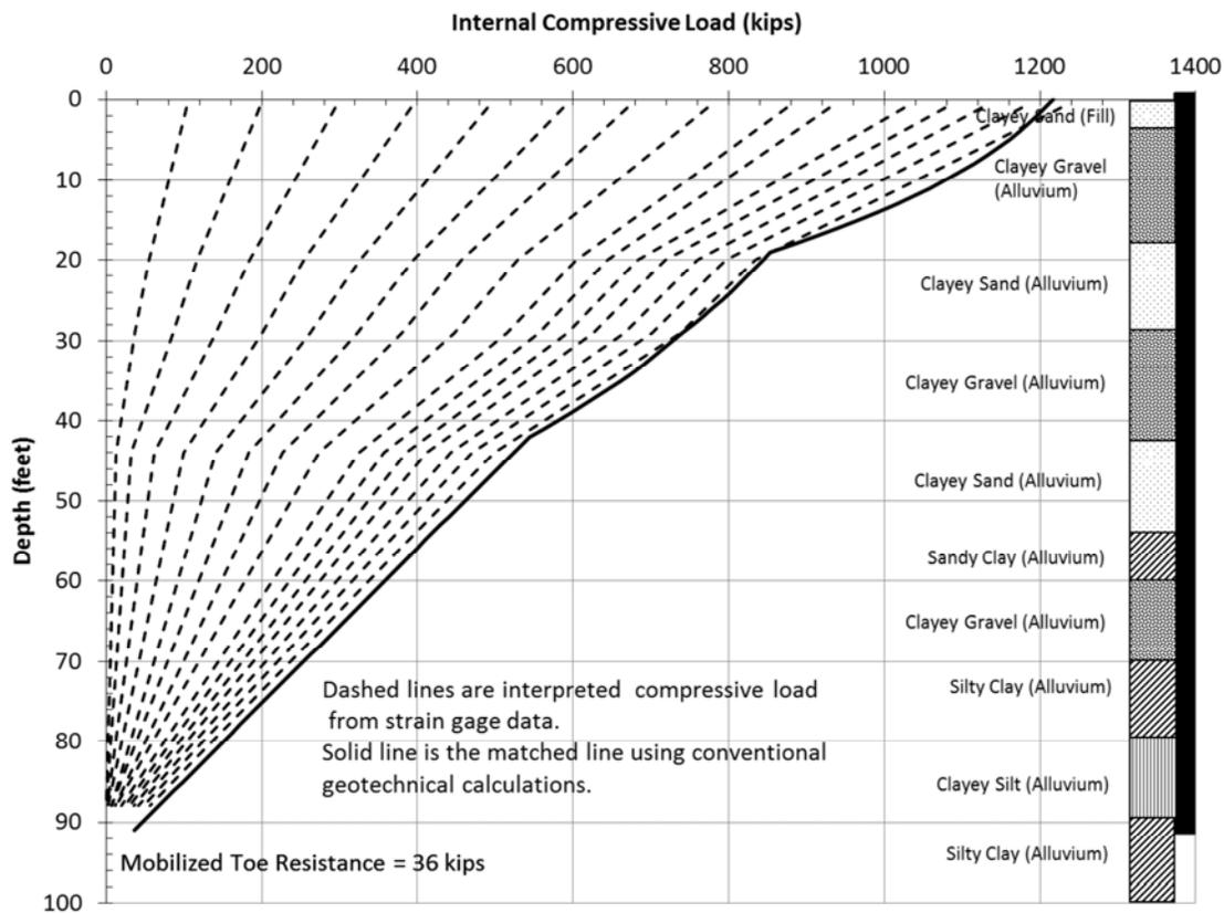
**FIG 6. Axial Compressive Load Distribution for Test Pile TP2**
