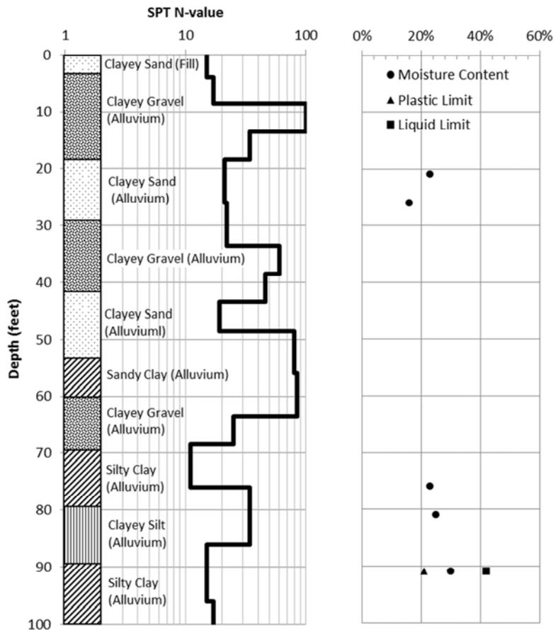
FIG 2. Typical test boring (1ft = 0.305m)
