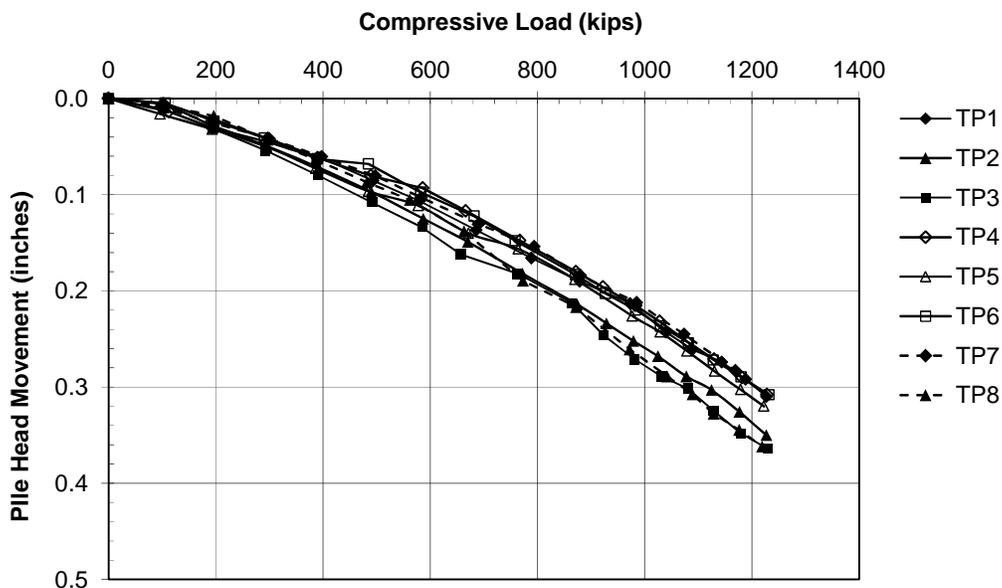
FIG 5. Pile Head Movement Versus Top Load (1 in = 25.4 mm, 1 kip = 4.45 kN)
