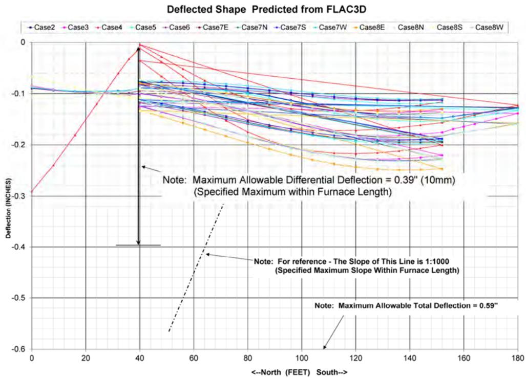
**FIG 4. Predicted Top of Concrete Alignment under All 14 Load Cases**
