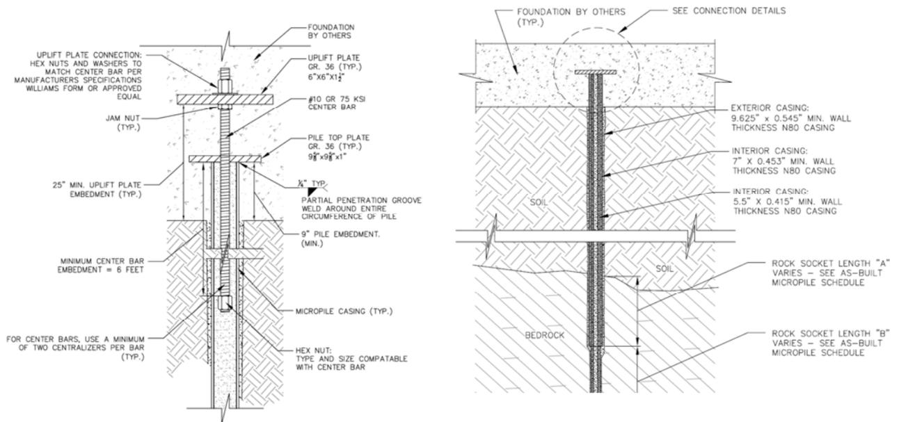
**FIG 6. Typical Micropile Designs**
