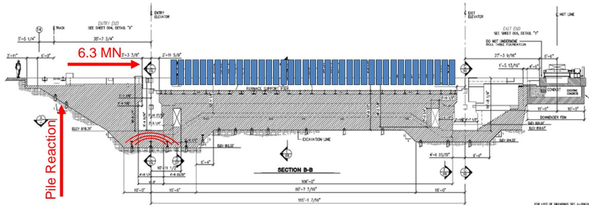
**FIG 3. Typical Section Through Furnace Foundation with Pusher Force**
