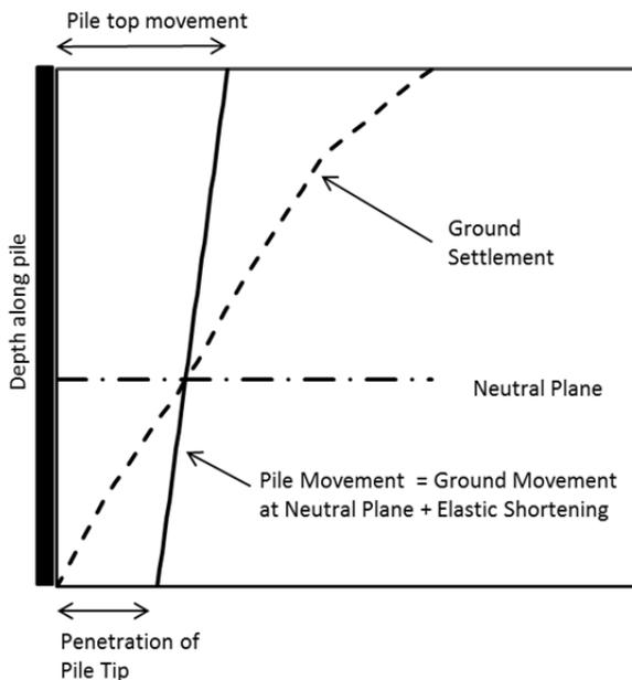
Figure 6. Ground settlement, pile movement, and neutral plane
