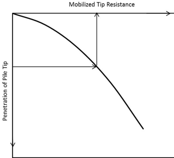
Figure 7. Pile tip penetration versus mobilized tip resistance
