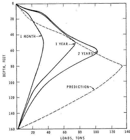
Figure 1. Compressive internal force distribution in 305mm dia. steel pipe pile (Crawford, 1969)
