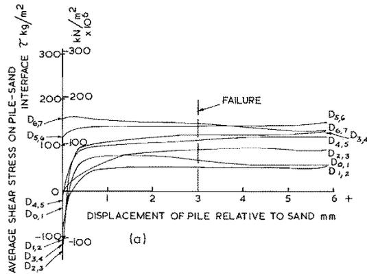
Figure 3. Development of shear stress along pile
