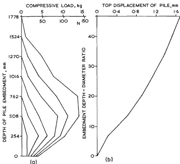
Figure 2. Compressive internal force distribution and pile top displacement during sand filling (Hanna and Tan, 1973)
