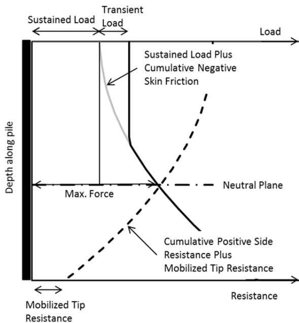
Figure 8. Neutral plane plot with transient load less than drag force
