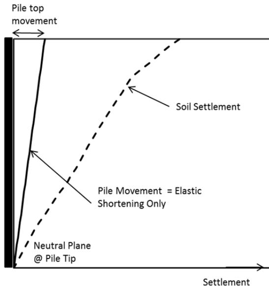
Figure 13. Ground settlement, pile movement, and neutral plane for example shown in Figure 11
