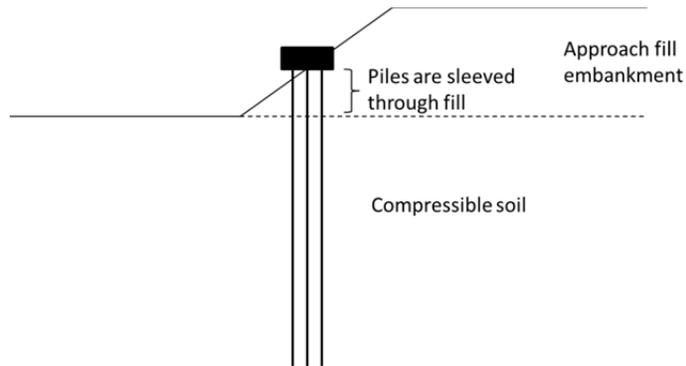
Figure 10. Piles through embankment fill supported in compressible soil
