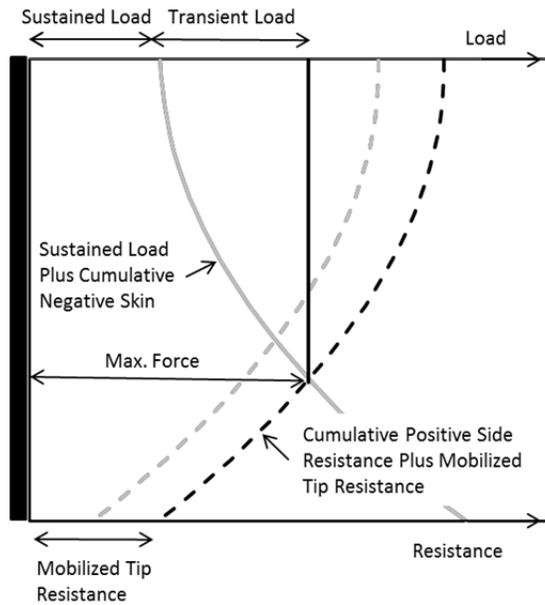
Figure 9. Neutral plane plot with transient load less than drag force
