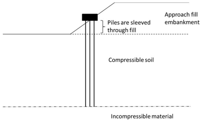
Figure 11. Piles through embankment fill supported on incompressible material
