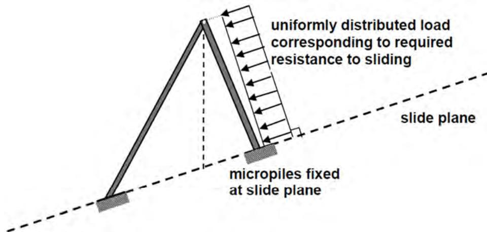
Figure 2. Plane frame model and assumed loading of micropile wall.
