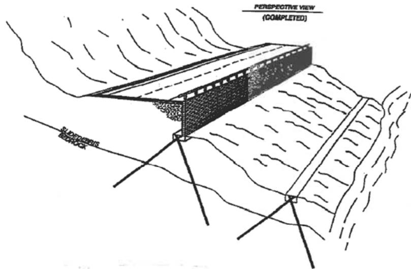
Figure 1. General Layout of Micropile Walls
