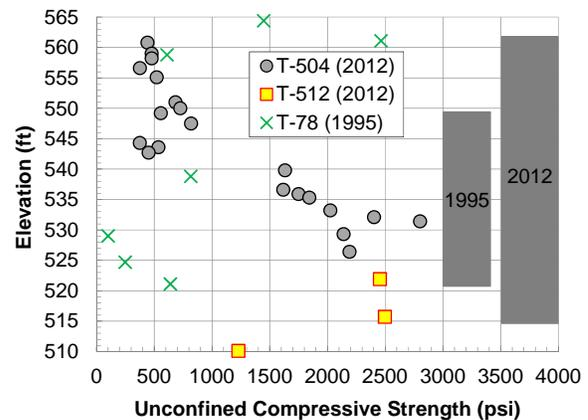
**Figure 5: Bedrock Core Strength.**
