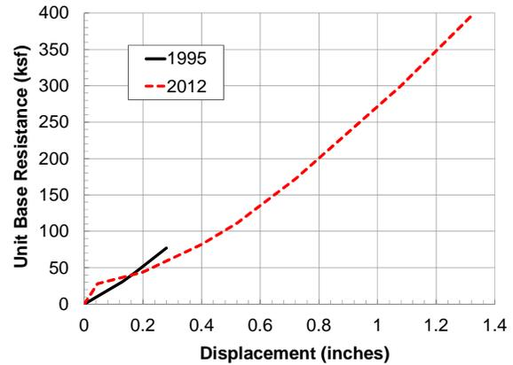
**Figure 9: Measured Unit Base Resistance.**
