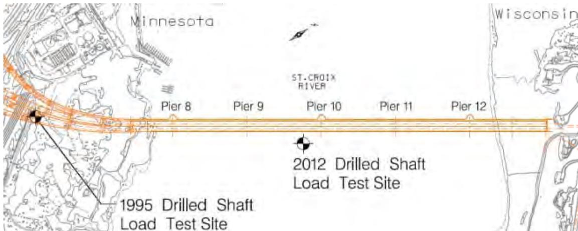
Figure 2: Test Shaft Locations.
