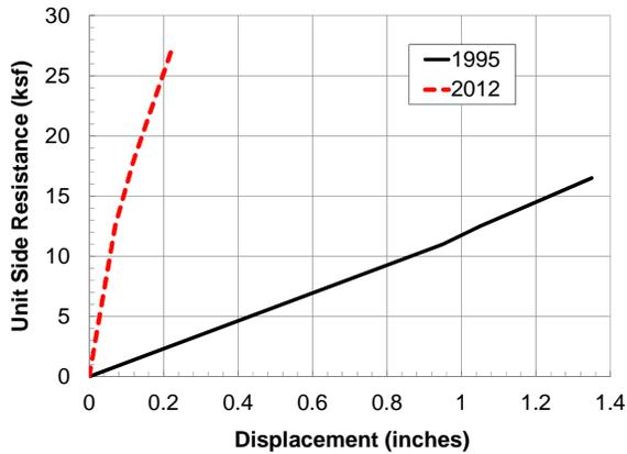
**Figure 8: Average Measured Unit Side Resistance in Rock Sockets.**
