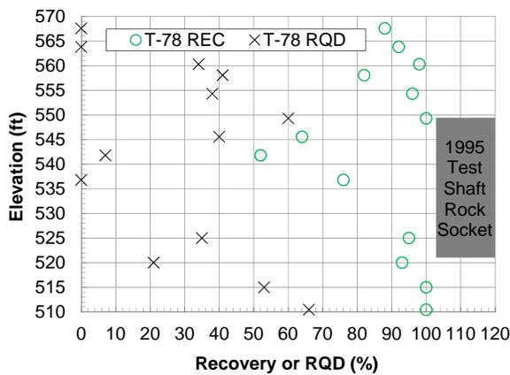
**Figure 3: 1995 Test Site Bedrock Core Information.**
