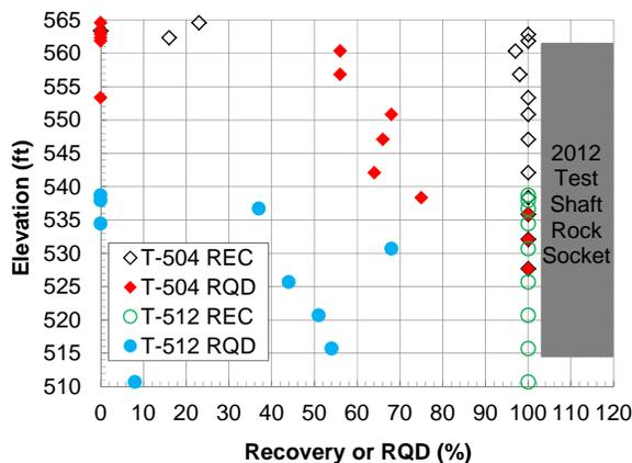
**Figure 4: 2012 Test Site Bedrock Core Information.**
