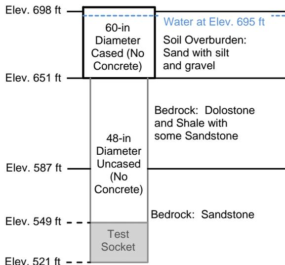
**Figure 6: 1995 Test Shaft Schematic.**
