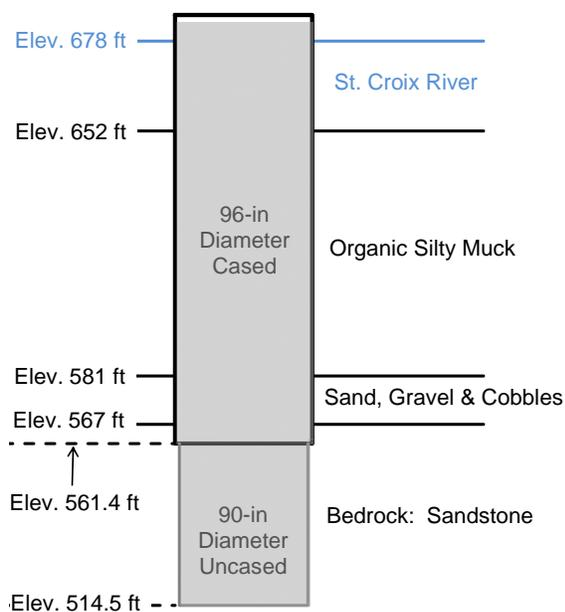
**Figure 7: 2012 Test Shaft Schematic.**
