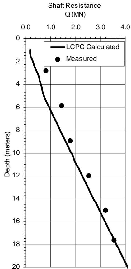
FIG. 10. Ultimate Shaft Resistance for S-4
