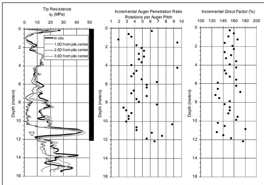
**Fig. 3 CPT and Installation Data for Test Pile S-2, D - 410 m (16 in)**
