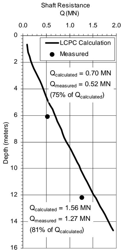
FIG. 9. Ultimate Shaft Resistance for S-3
