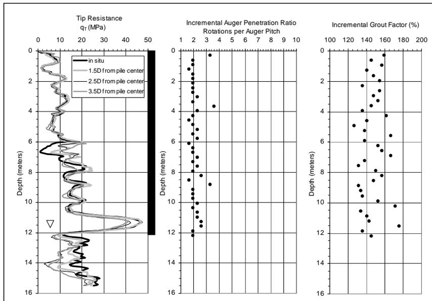
**Fig. 2 CPT and Installation Data for Test Pile S-1, D - 410 m (16 in)**
