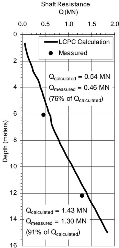
FIG. 7. Ultimate Shaft Resistance for S-1
