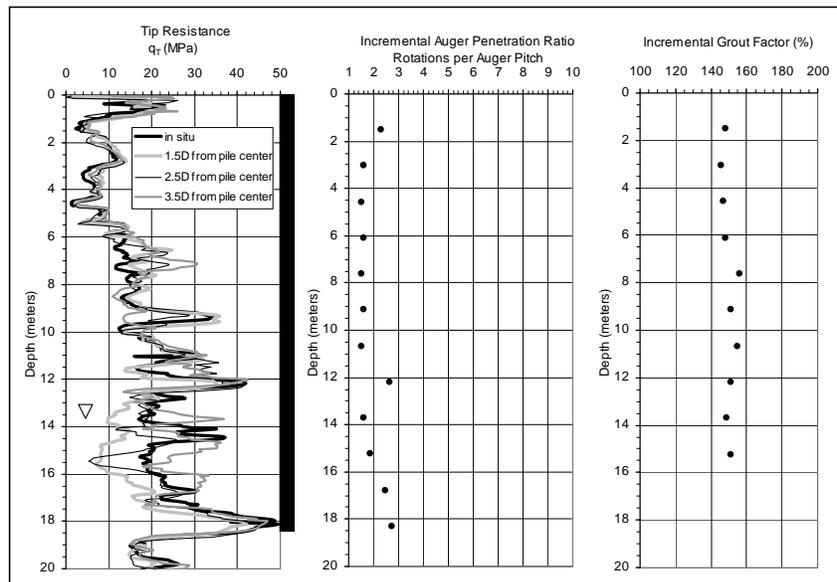
**Fig. 5 CPT and Installation Data for Test Pile S-4, D - 410 m (16 in)**
