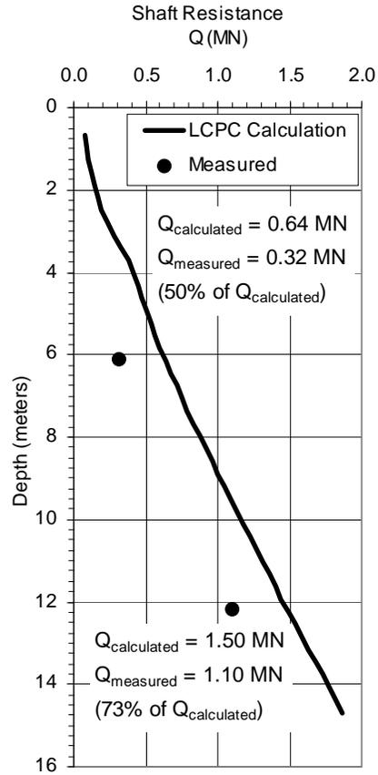
FIG. 8. Ultimate Shaft Resistance for S-2
