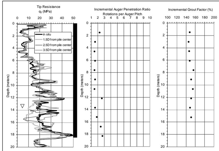
**Fig. 4 CPT and Installation Data for Test Pile S-3, D - 410 m (16 in)**
