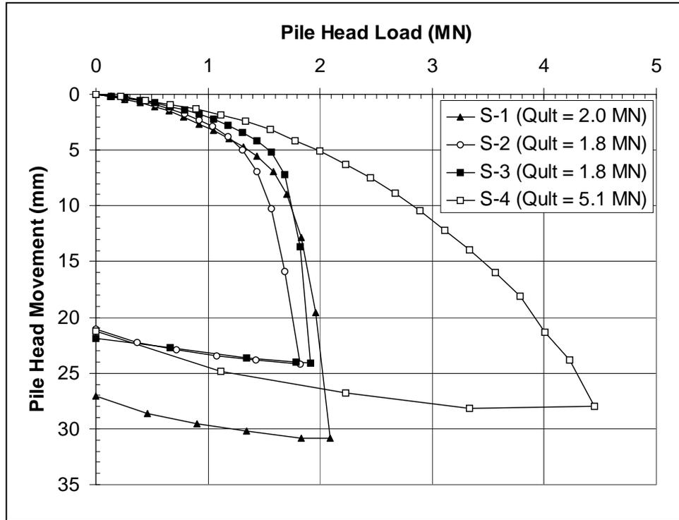
Fig. 6 Pile Head Load-Movement from Test Piles
