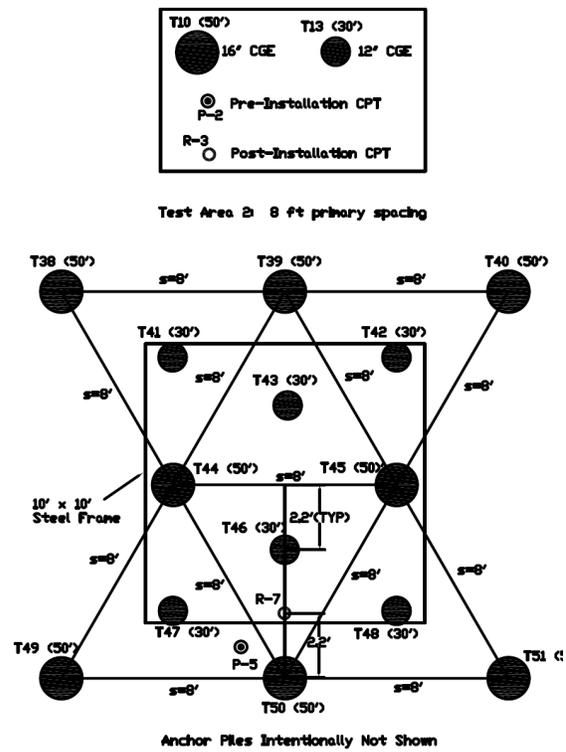
Figure 4. Set Up of Large Plate Test 2
