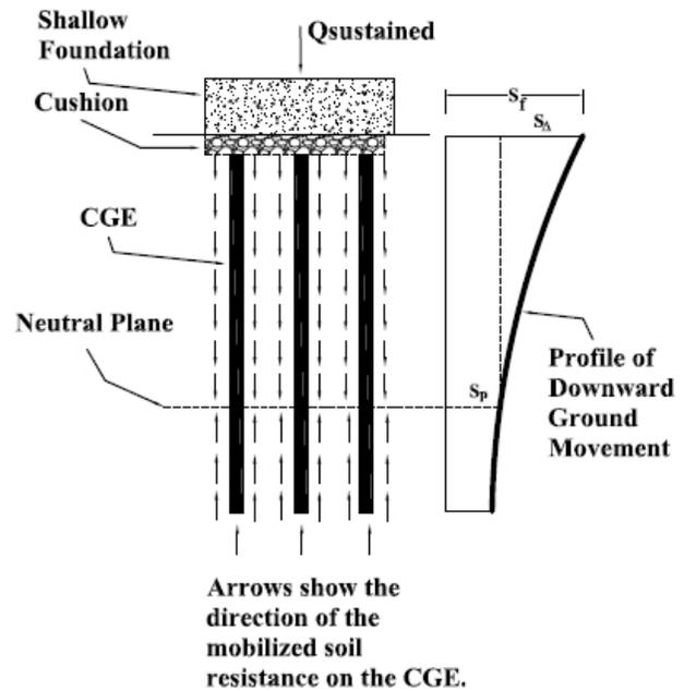
**Figure 12. Conceptual Settlement Model of Composite Ground**
