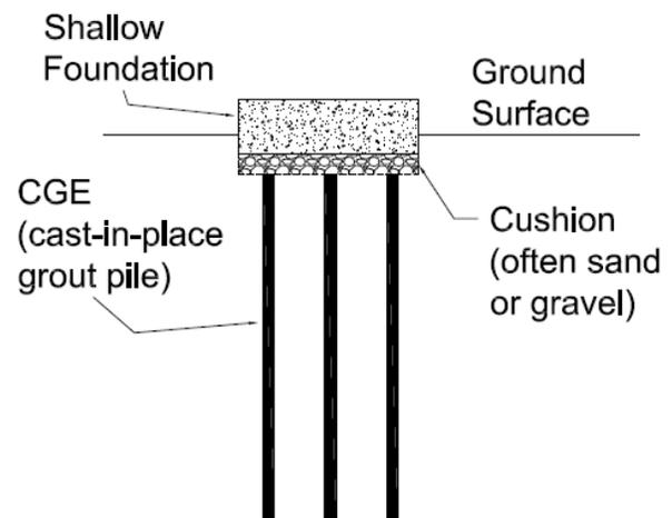
Figure 1. Composite Ground with CGEs
