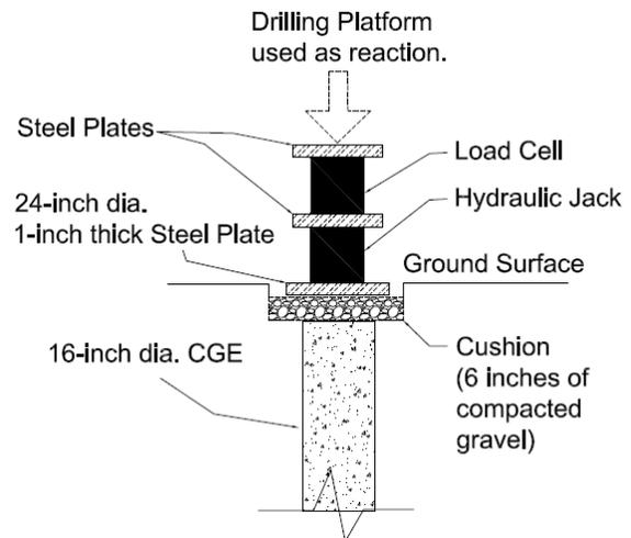
Figure 2. Small Plate Test Setup
