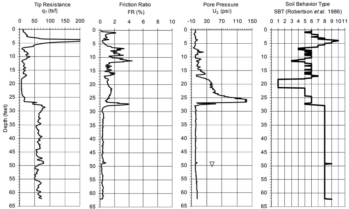
**Figure 7. Cone Penetration Test Data for Project Site**
