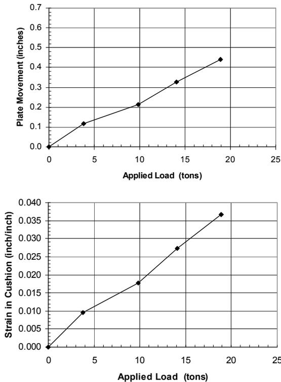
**Figure 8. Small Plate Test Results**
