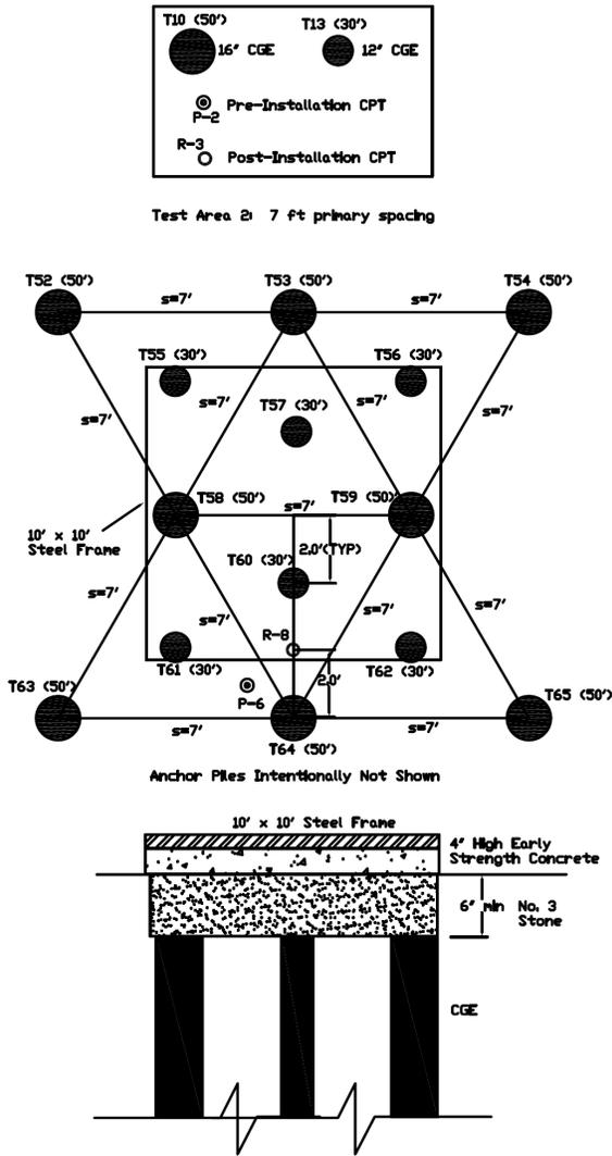
Figure 5. Set Up of Large Plate Test 3
