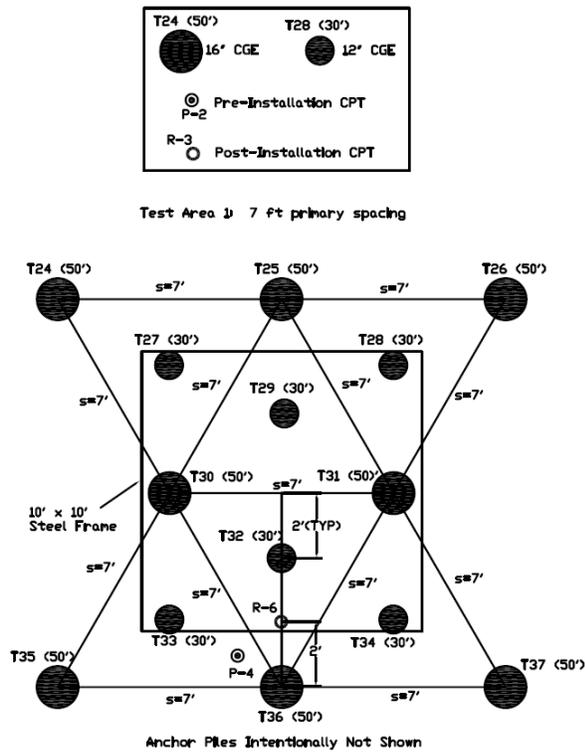
Figure 3. Set Up of Large Plate Test 1
