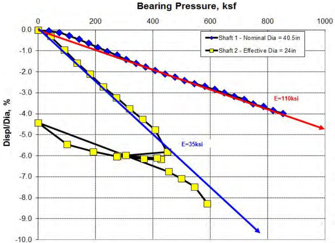
**Figure 8** Unit Base Resistance vs. Normalized Downward Displacement of O-Cell (Lawrenceville Site)
