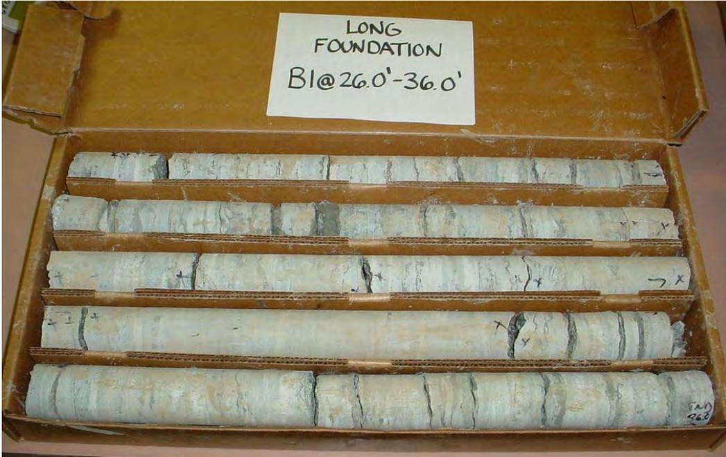
**Figure 1** Rock Core from Nashville Boring B-1, Location of Test Shaft 1
