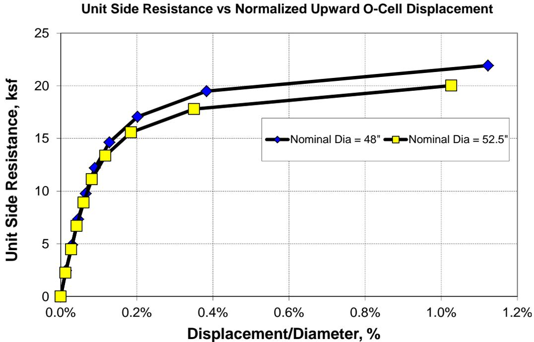
**Figure 3** Average Unit Side Resistance vs. Normalized Upward O-Cell Displacement (Nashville Site)
