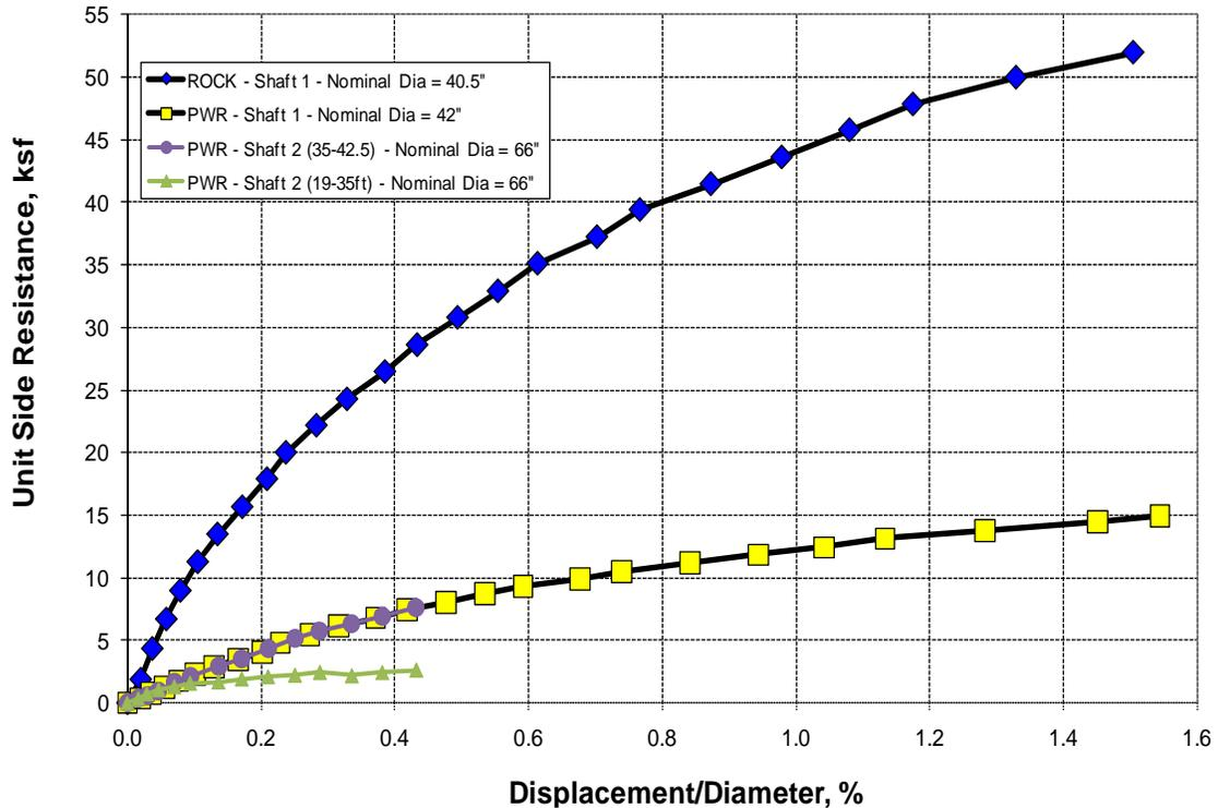
**Figure 7** Average Unit Side Resistance vs. Normalized Upward O-Cell Displacement (Lawrenceville Site)
