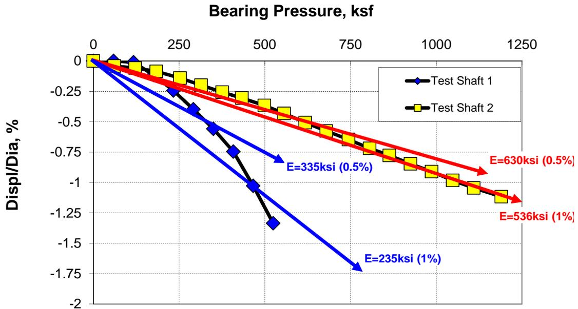
**Figure 4** Unit Base Resistance vs. Normalized Downward Displacement of O-Cell (Nashville Site)
