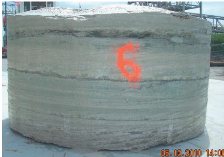
[FIG. 9] Core Run 6 from Test Shaft Excavation
