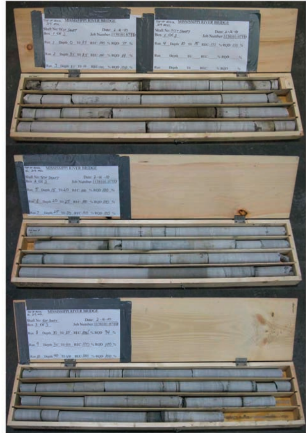
[FIG. 3] Test Shaft Boring Recovered Rock Core
