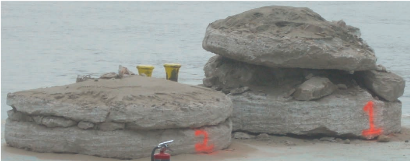
[FIG. 7] Core Runs 1 and 2 from Test Shaft Excavation
