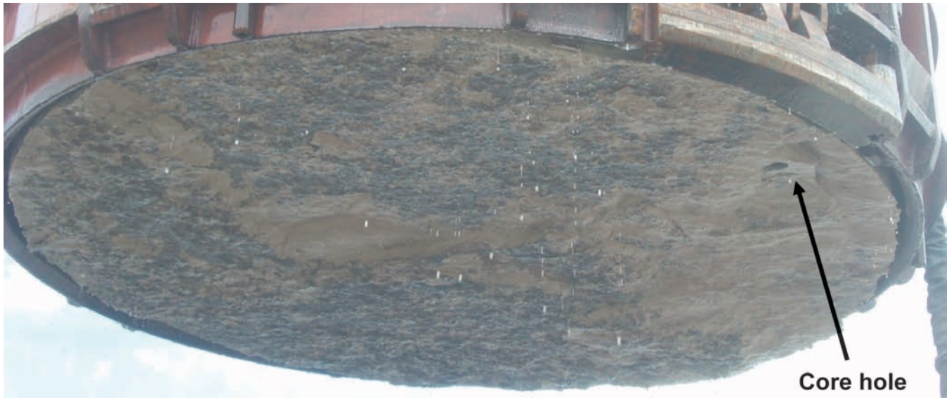
[FIG. 10] Bottom of Core Run 6 from Test Shaft Excavation
