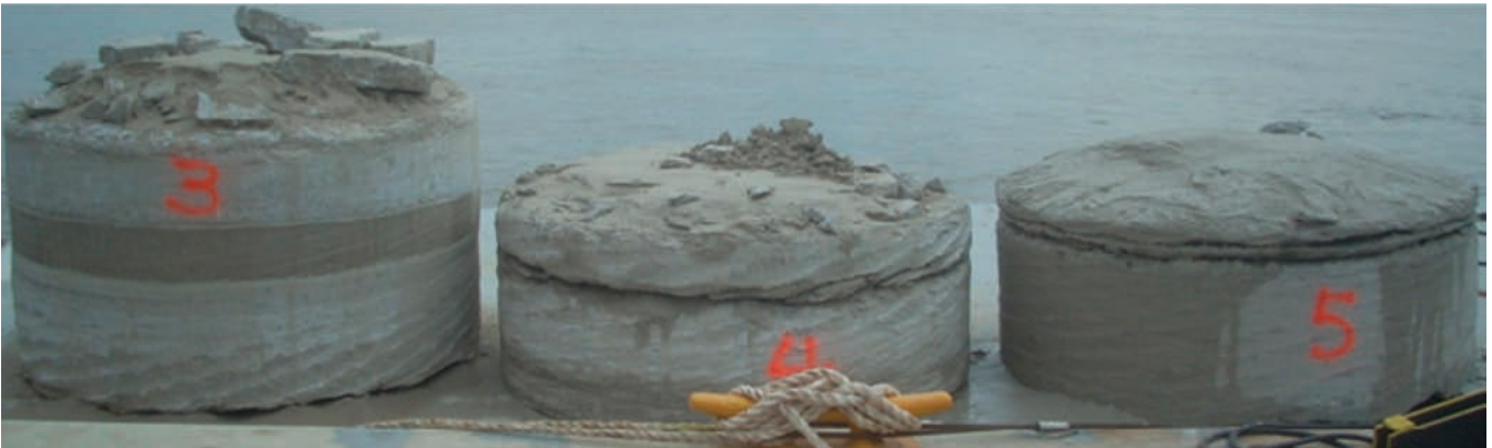
[FIG. 8] Core Runs 3 through 5 from Test Shaft Excavation
