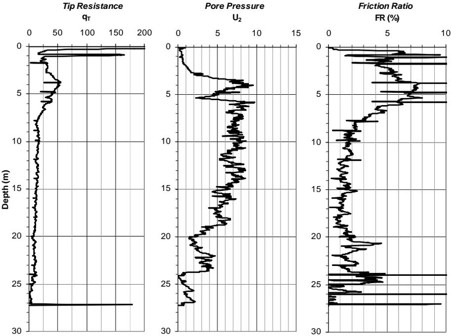
**Figure 2. CPT Profile for Example Site No. 2.**
