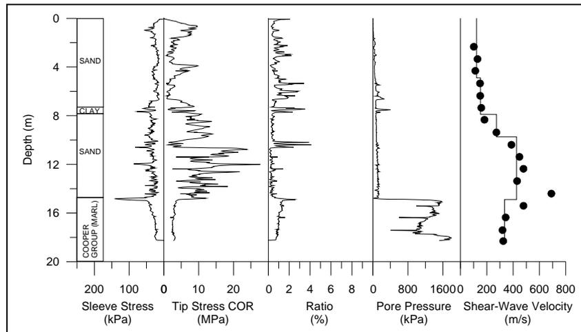
Figure 2. Characteristic Sand Profile
