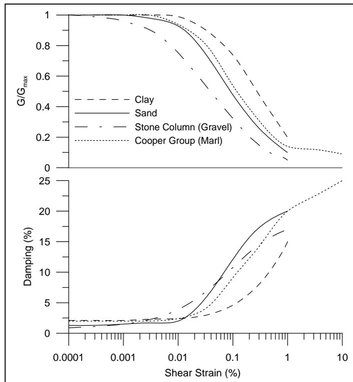
Figure 3. Modulus Reduction and Damping Curves
