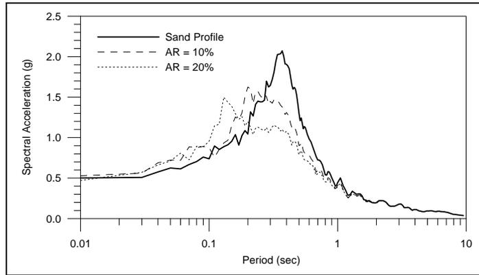
Figure 6. Acceleration Response Curves for Sand
