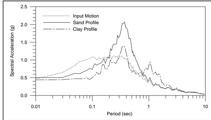
Figure 4. Acceleration Response Curves for Unimproved Soil
