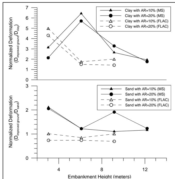
Figure 8. Normalized Horizontal Embankment Deformation
