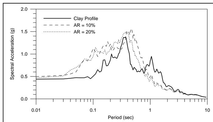
Figure 5. Acceleration Response Curves for Clay
