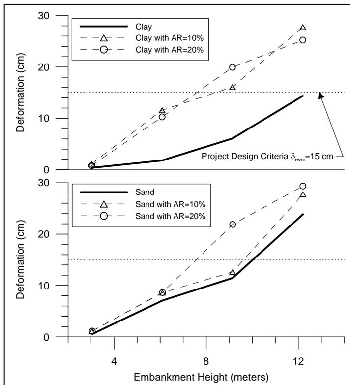
Figure 7. Horizontal Embankment Deformation
