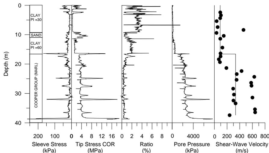
Figure 1. Characteristic Charleston Profile with Clay Overburden.
