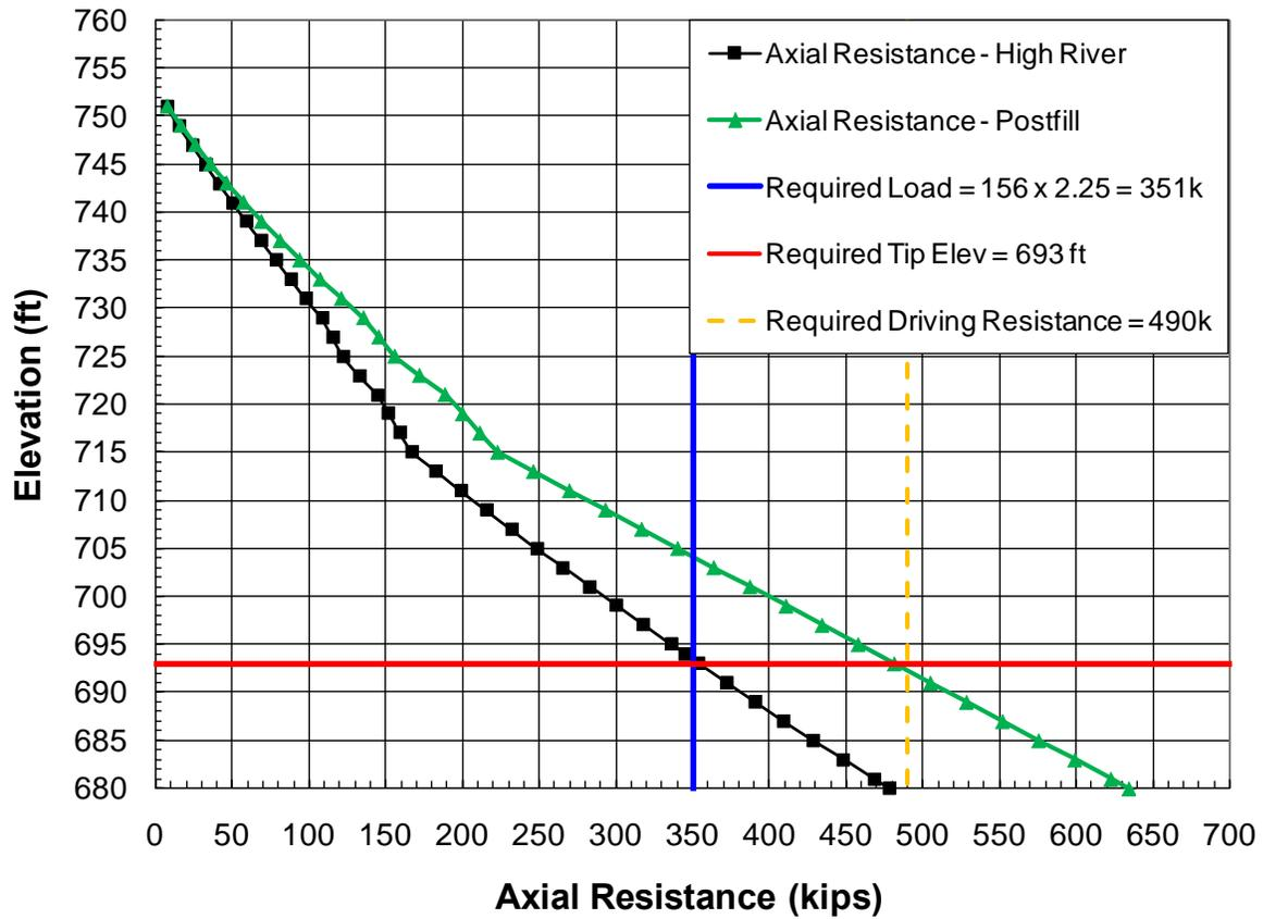
Figure 1: Axial Resistance for HP14x73 Piles at the North End Bent
