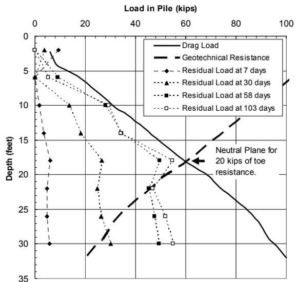
**Figure 5. Residual Load Distribution Interpreted from Strain Gages**
