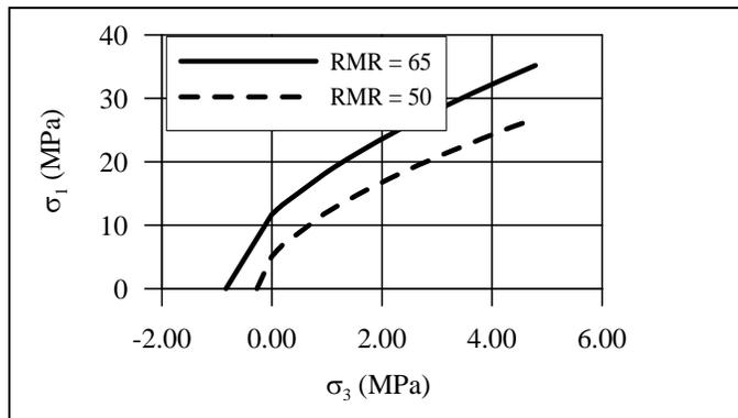
Figure 1: Site-Specific Hoek-Brown Failure Criterion
