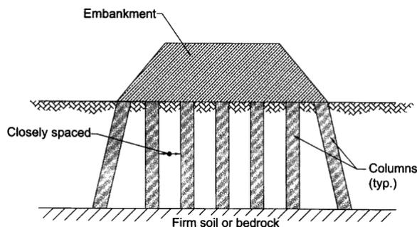
Figure 1. Column-supported embankment (after Collin, 2004)
