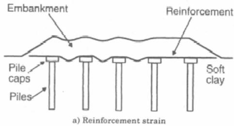
Figure 5. Reinforcement strain limit-state failure from BS 8006
