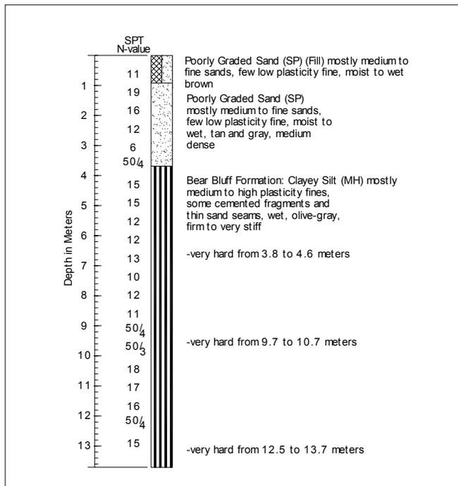
Figure 1 Typical Test Boring Record
