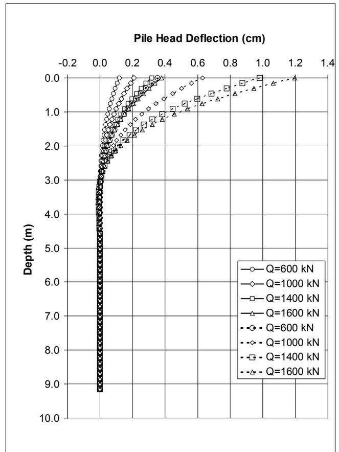
Figure 4 Lateral Deflection of Pile Model
