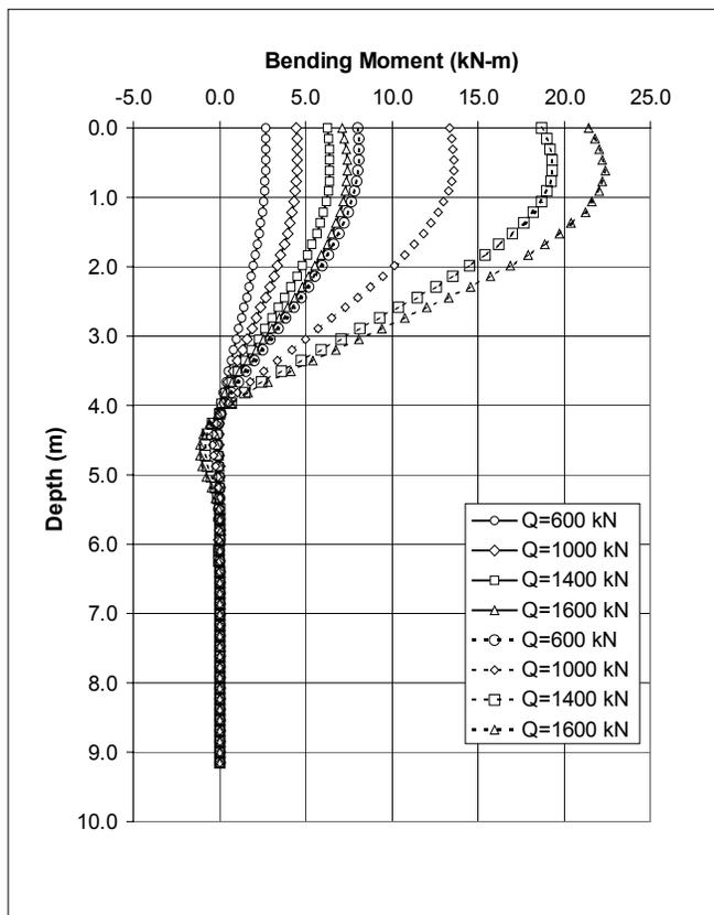
Figure 6 Bending Moment in Pile Model
