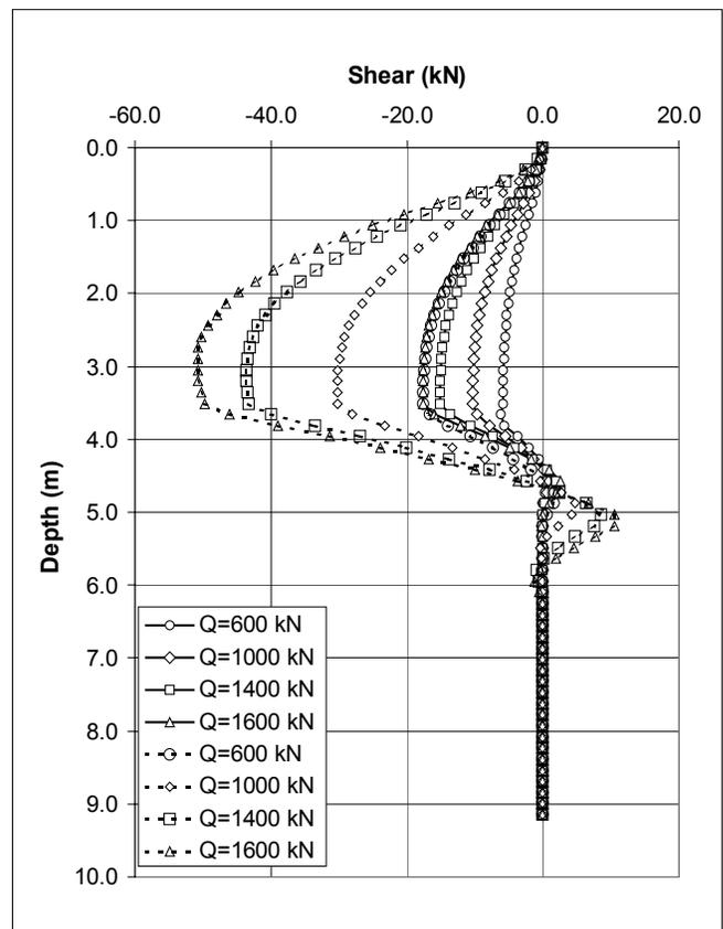
Figure 5 Shear in Pile Model
