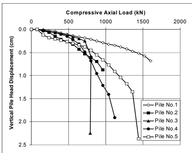
Figure 3 Load versus Pile Head Displacement
