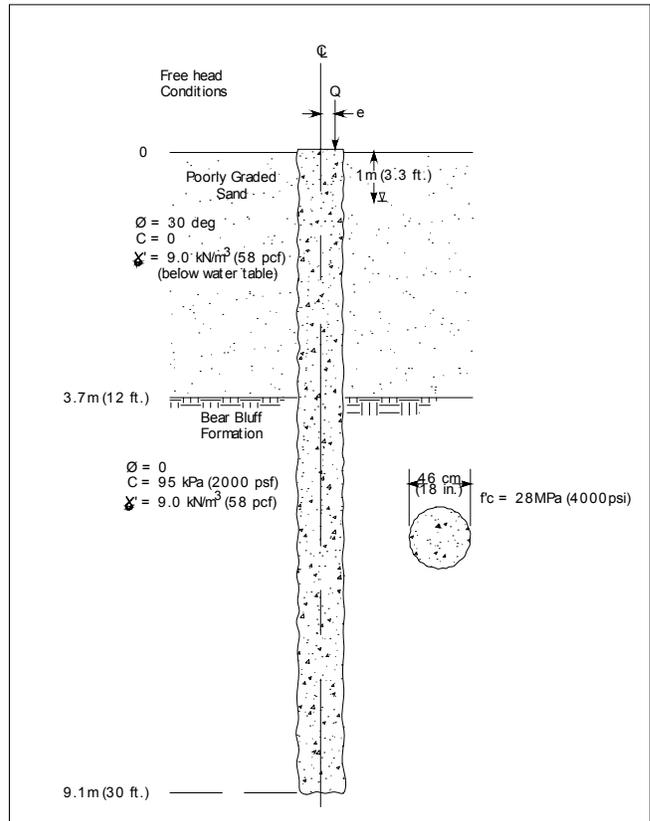
Figure 2 Idealized Sketch of Cast-In-Place Pile
