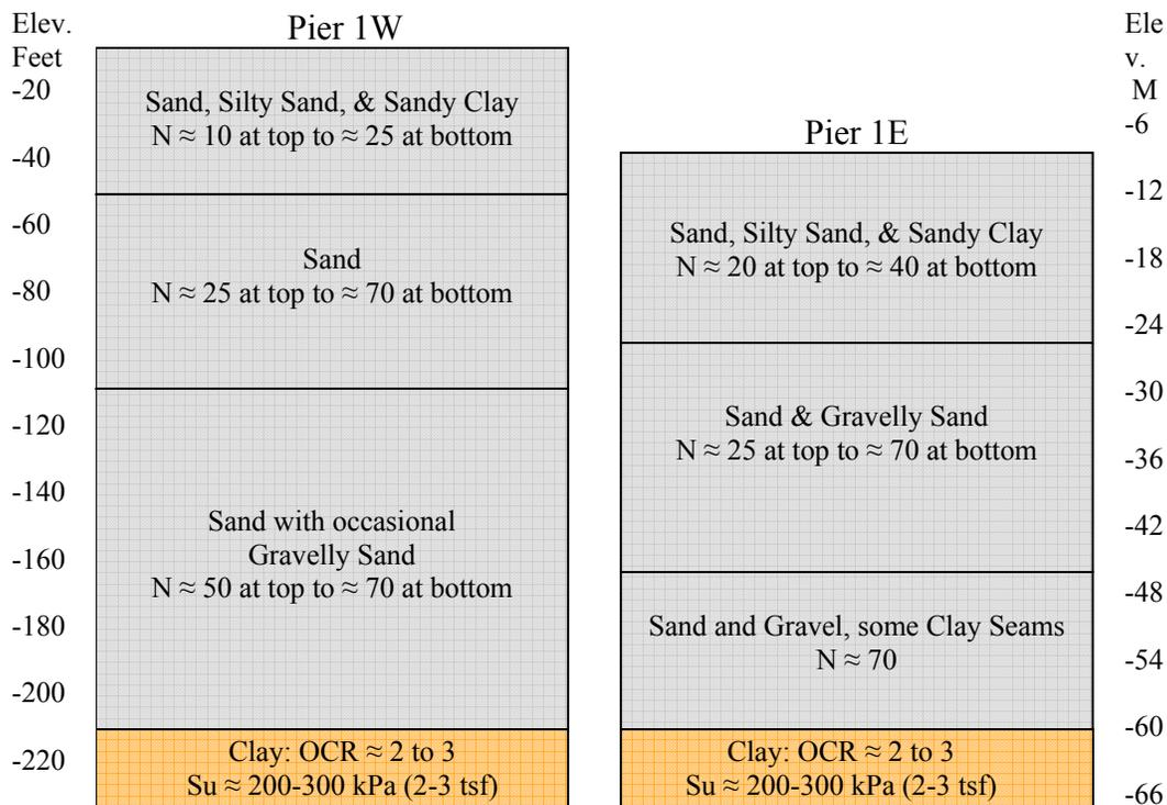
Figure 1. Soil Stratigraphy and Pertinent Geotechnical Properties
