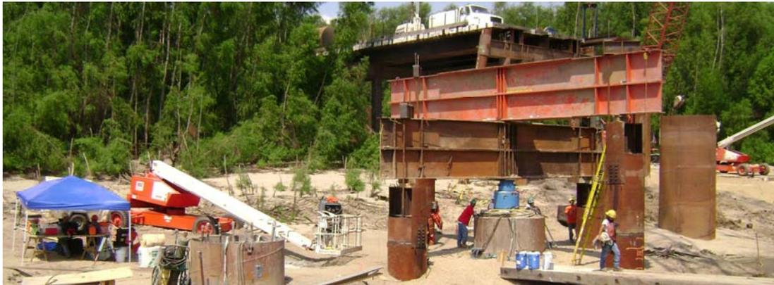
**Figure 4. Top of Shaft Reaction Frame to Supplement Upward Resistance against Base Resistance during O-cell Testing.**
