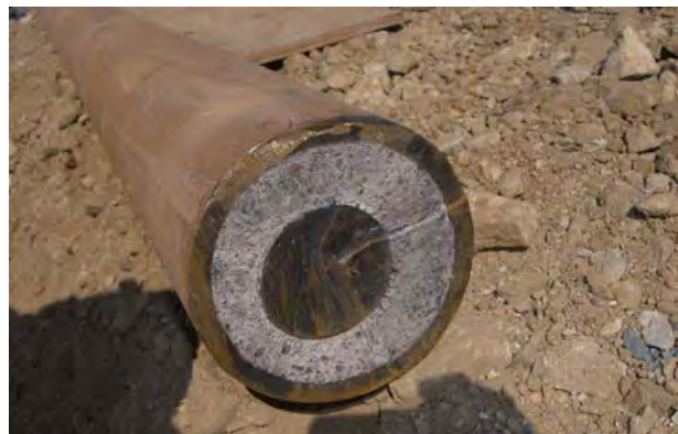
Figures 4a and 4b: Photographs of Faulty Micropiles following Extraction
