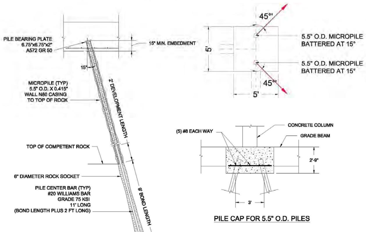
**Figure 3. Micropile Detail and Layout for Condominiums, Knoxville, Tennessee
