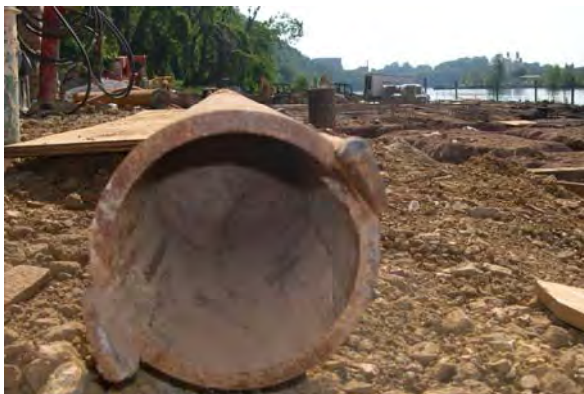
Figures 4a and 4b: Photographs of Faulty Micropiles following Extraction
