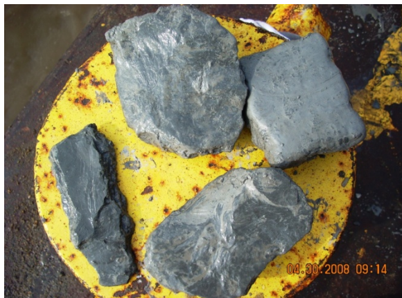
Figure 3: Shale recovered from drilling bucket at tip of test shaft.
