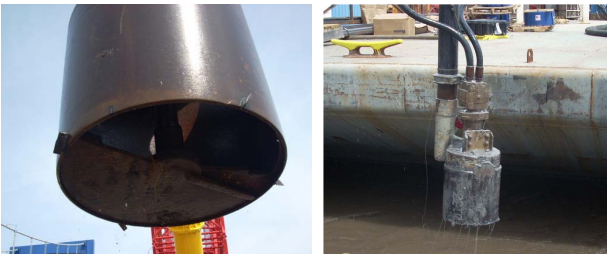
Figure 10: Test shaft clean-out tools: one-eyed bucket and hydraulic pump
