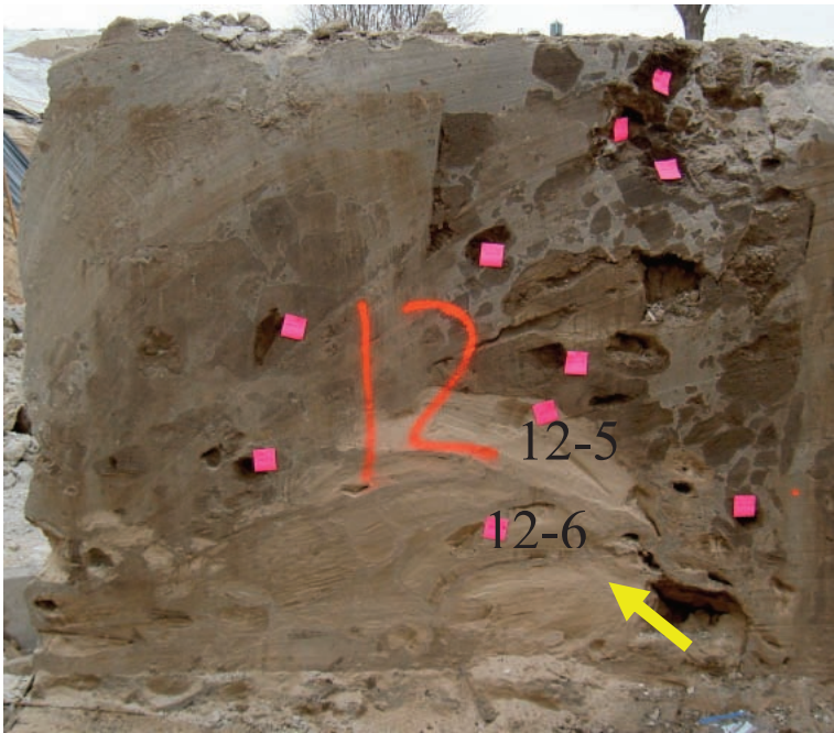
[FIG. 12] Soil inclusions in triple fluid jet grout column #12.
