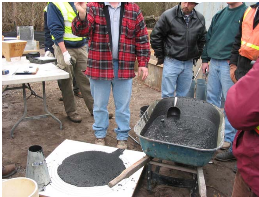
Figure 1 Slump Flow Test on SCC (Concrete is Colored Black)
