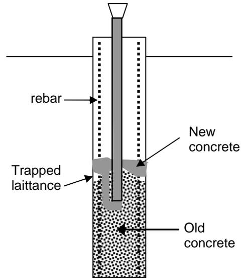
Figure 1 Loss of Workability in Tremie Placed Concrete
