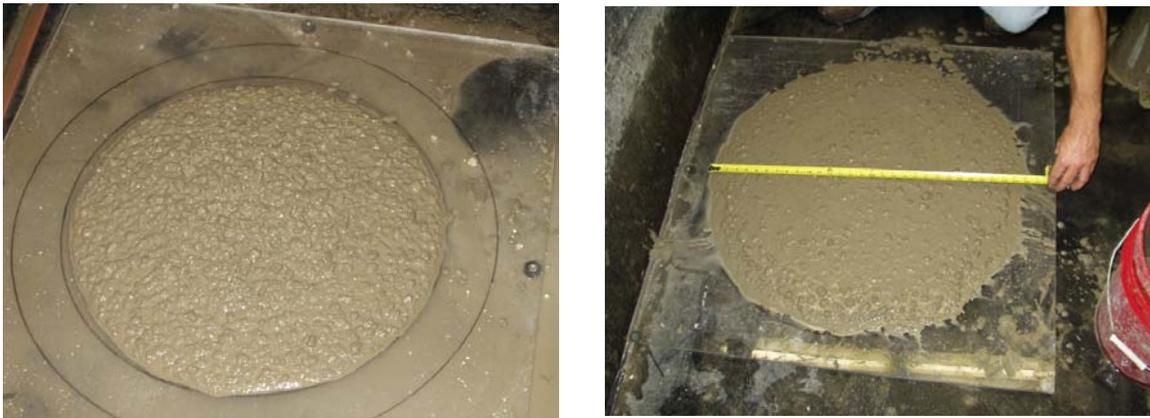
Figure 4 SCC Mixes, with cohesive paste (left) and segregation (right)
