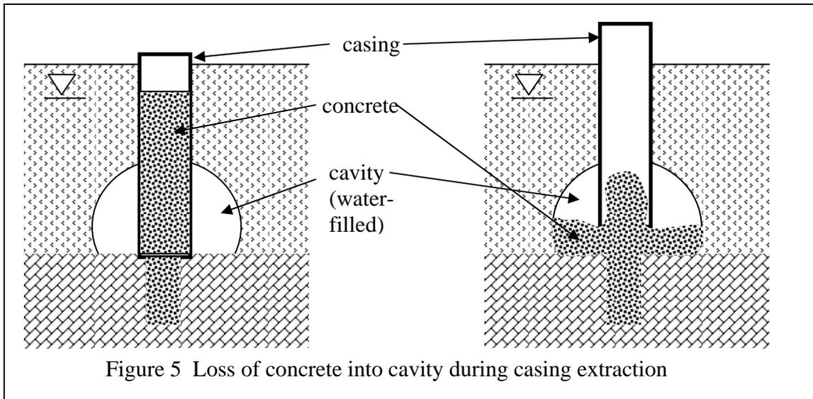
could result in the head of concrete within the casing becoming less than the head of water on the outside of the casing. If this condition occurs, there will be flow of water into the casing, potentially displacing or mixing with the concrete.
