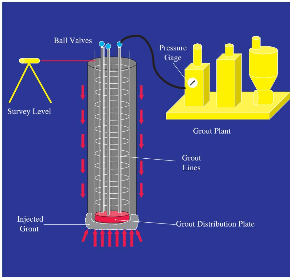
*Pumping high pressure grout below the base of the shaft through a specially designed distribution system allows the end bearing capacity of drilled shafts to be greatly enhanced and provides unparalleled quality assurance on every shaft.*
