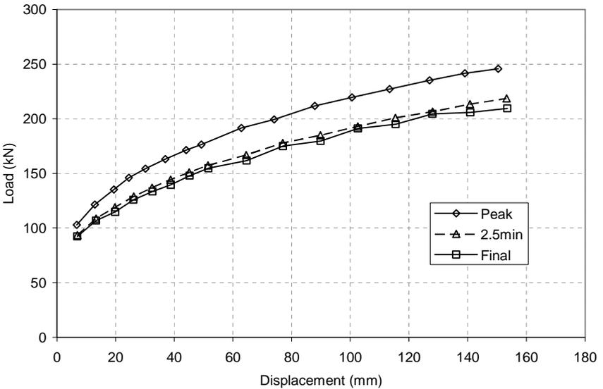
FIG. 2b. Shaft BS peak, 2.5 minute and final load versus displacement.
