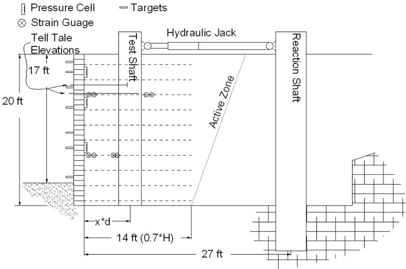
**FIG. 1 Sketch of Shaft B and instrumentation locations.**
