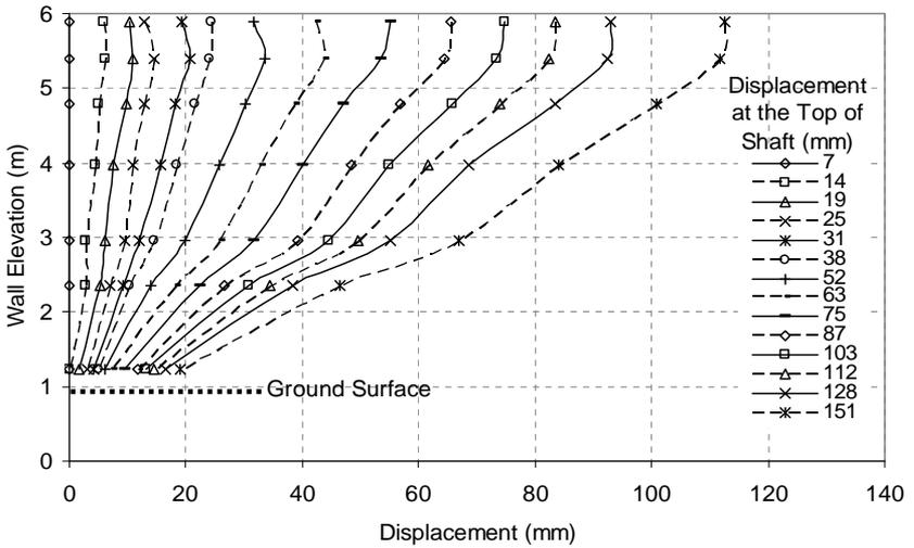
FIG. 4a. Wall facing displacement for Shaft B.
