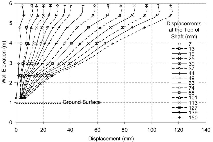
FIG. 4b. Wall facing displacement for Shaft BS.
