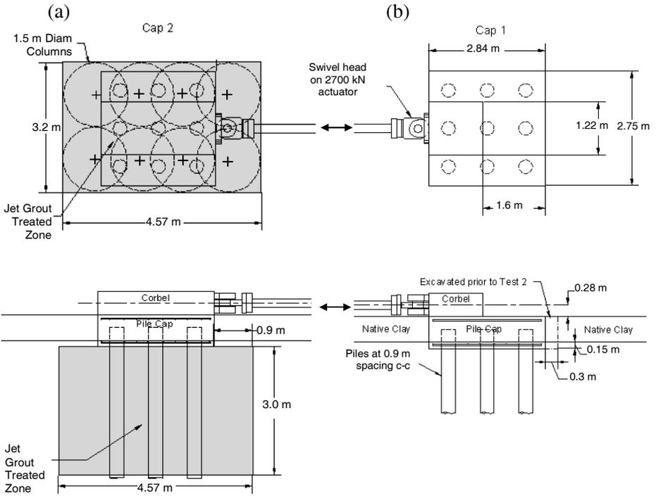
**FIG. 2. Plan and profile drawings of the pile group (a) after jet grout treatment and (b) in virgin clay before jet grout treatment.**
