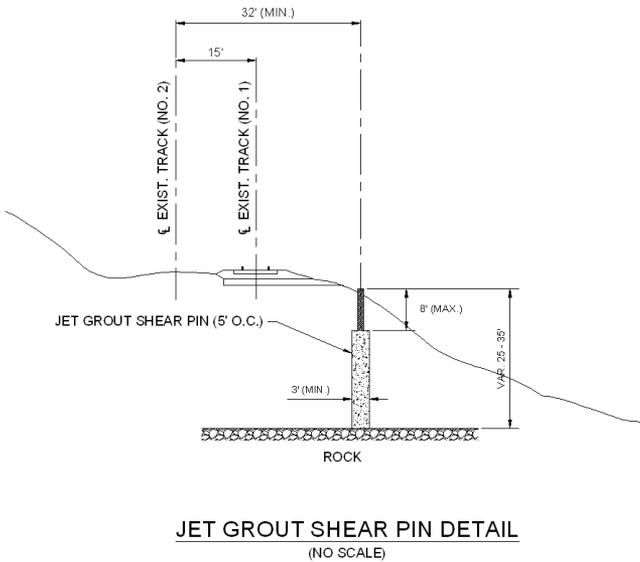
**FIG. 2. Proposed Jet-Grout Shear Pin Detail**
