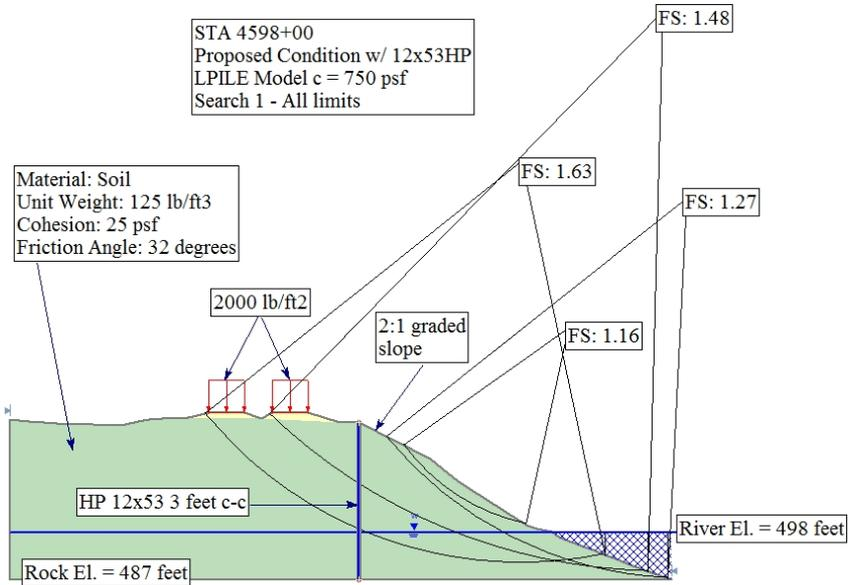
**FIG. 4. Typical Result from Analysis of Embankment Stabilized Using H-Piles**
