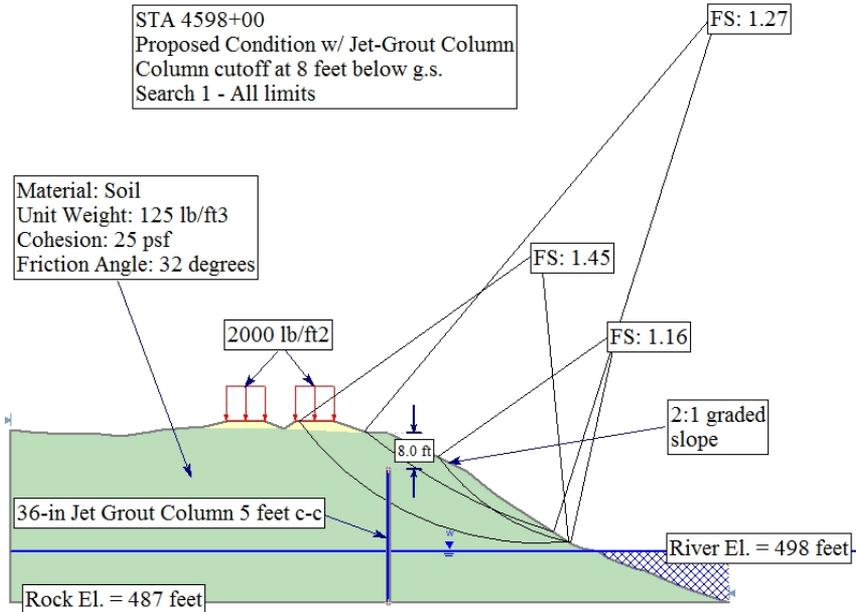
**FIG. 5. Typical Result from Analysis of Embankment Stabilized Using Jet-GROUT Columns**
