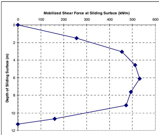
**FIG. 3. Predicted Shear Resistance at Sliding Surface for H-Piles subjected to Soil Movement of 127 mm (5 inches)**
