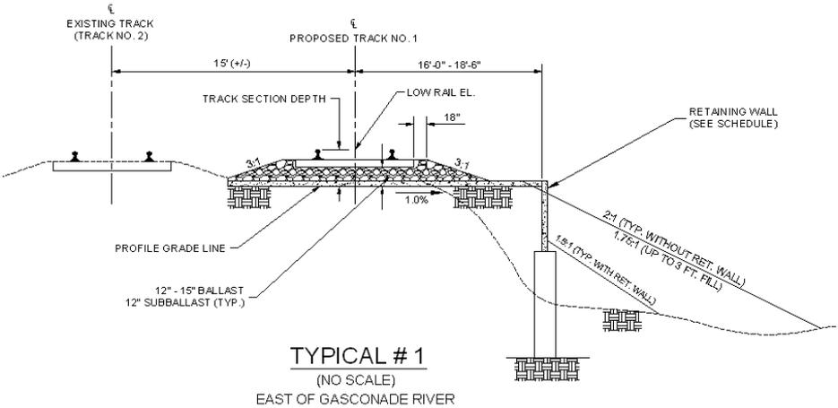
**FIG. 1. Typical Cross-Section of Project Alignment (Retaining Wall Shown)**
